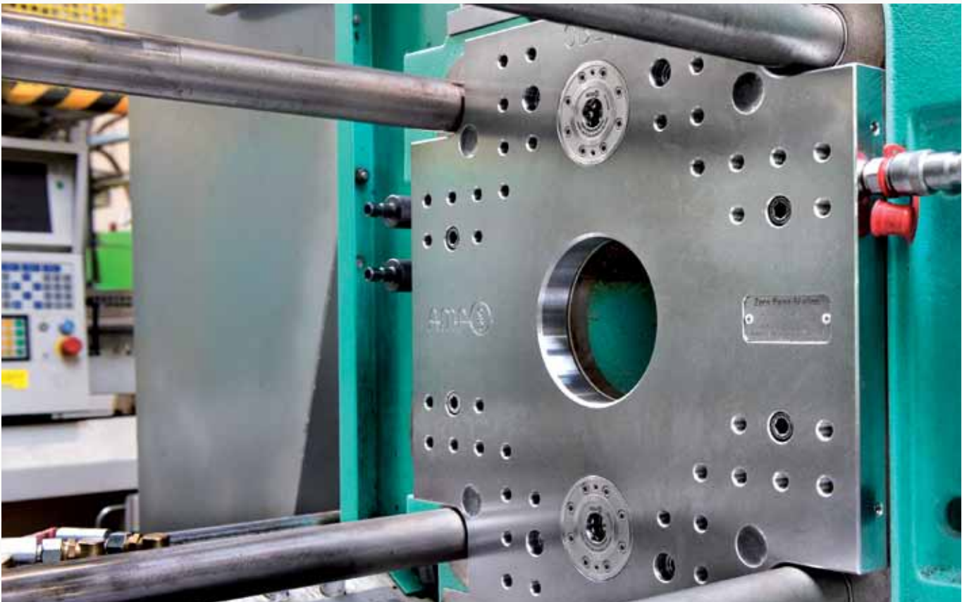
In injection moulding, the tools are successfully changed in a way that optimizes set-up time through the use of the AMF Zero-Point System. With friendly recommendation of Robert Bosch GmbH, Waiblingen
