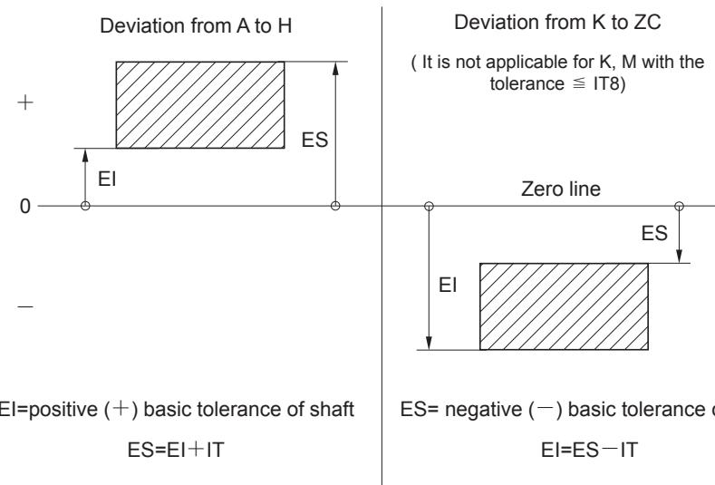
For example: for a hole with diameter 3 mm and tolerance H7, we can find that the lower deviation  $EI=0$  in relation to H7 from the basic tolerance table, and the standard tolerance  $IT=10\mu m$  corresponding to H7, thus the upper deviation  $ES=EI+IT=10\mu m$ . Therefore the hole fitting dimension is  $\emptyset 3^{+0.01}_0$  mm.
