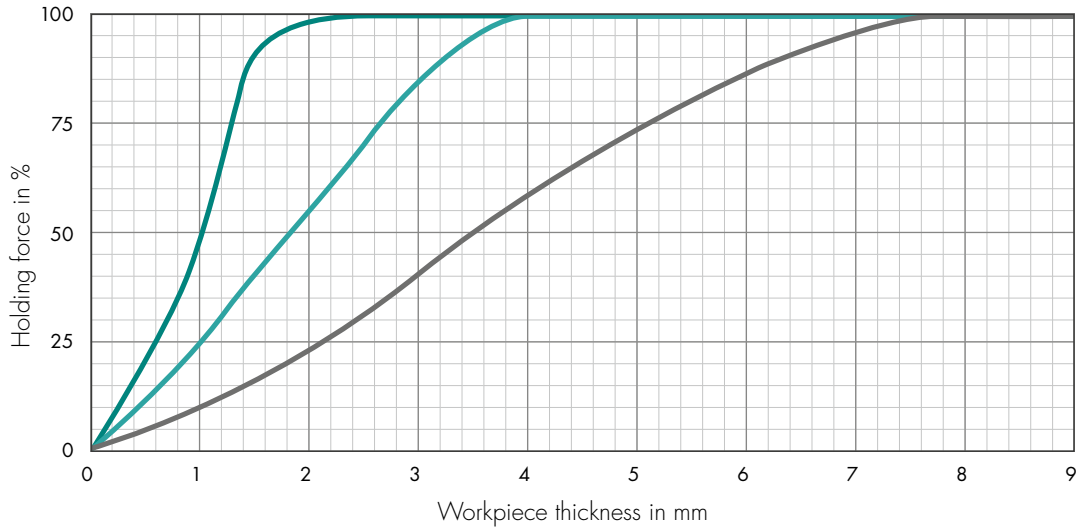
SAV 244.72 min. thickness of workpiece for circular magnets with ring pole pitch 5.5/9/18 mm
