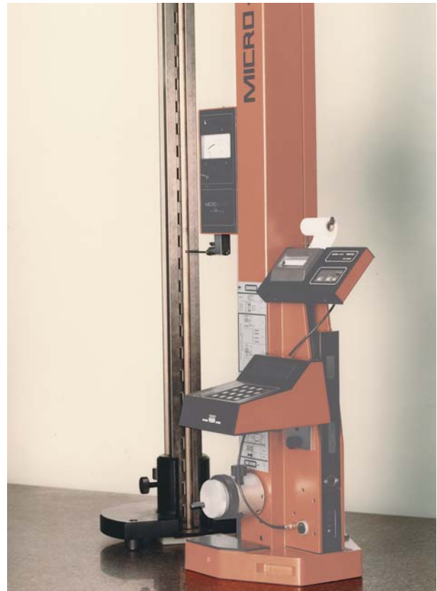
Fig. 12: KOBA-step aligned vertically for checking height gauges.
