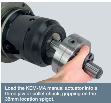
Actuate the power chuck to ensure KEM-MA is locked in position, adjust T.I.R as required.
