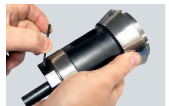
Lock stopper shaft and install
