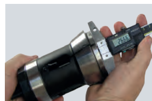
Adjust stopper shaft position
