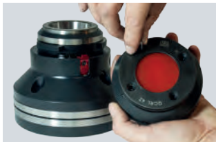
Remove bar seal from housing
