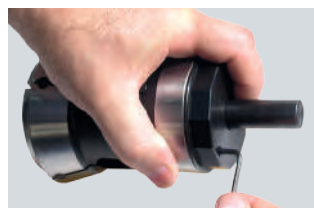
Lock stopper housing in position
