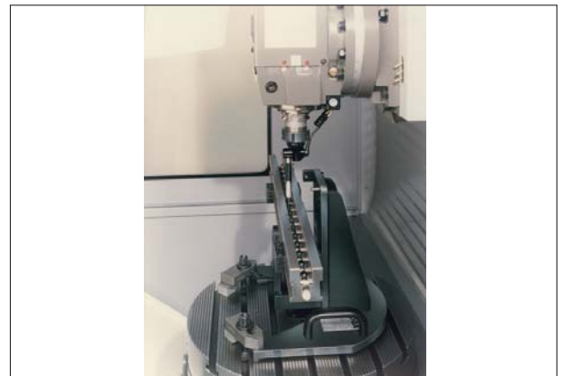
Fig. 18: KOBA-step, shown here installed on a flexible machining center for verifying its positioning accuracy (the center's dimensional-gauging head is integrated into its tool chuck).
