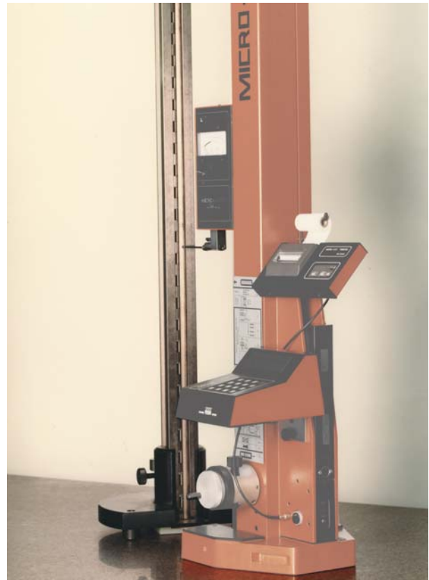
Fig. 12: KOBA-step aligned vertically for checking height gauges.
