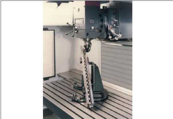
Fig. 15: KOBA-step installed on a swivel support and base, shown here spanning the major diagonal of the workspace of a vertical milling machine equipped with a dimensional-gauging head.
