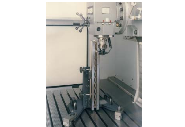
Fig. 17: KOBA-step, shown here aligned vertically for checking the Z-axis of a machine tool equipped with a dimensional-gauging head.
