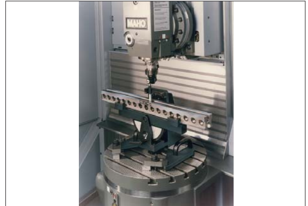
Fig. 16: KOBA-step, shown here horizontally aligned along the X-axis of the rotary bed of a machine tool equipped with a dimensional-gauging head.
