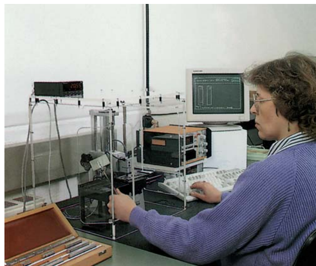
Gauge Block Inspection ▽
