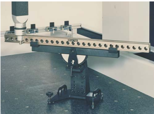
Fig. 9: Koba-step aligned horizontally along the XY-diagonal plane, same accessory as above, turned round 90°, stylus probe horizontal; Contacting through crossdrills.
