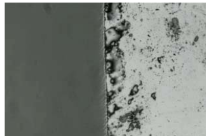
Magnification 500 x: CVD-Thickfilm-Diamond, Laser processing
