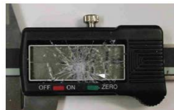
Competitor Product: after 100g weight fallen from 200mm height
