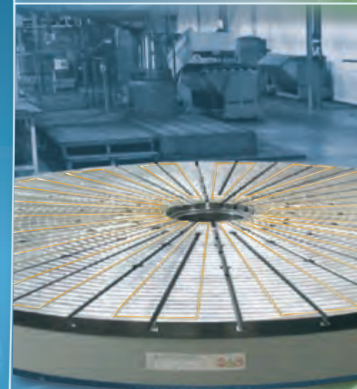
Grinding of large bearing rings Ø 2800 mm
