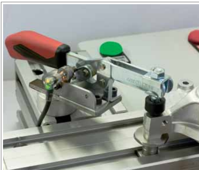
Horizontal toggle clamp with sensor monitoring for automation solutions
