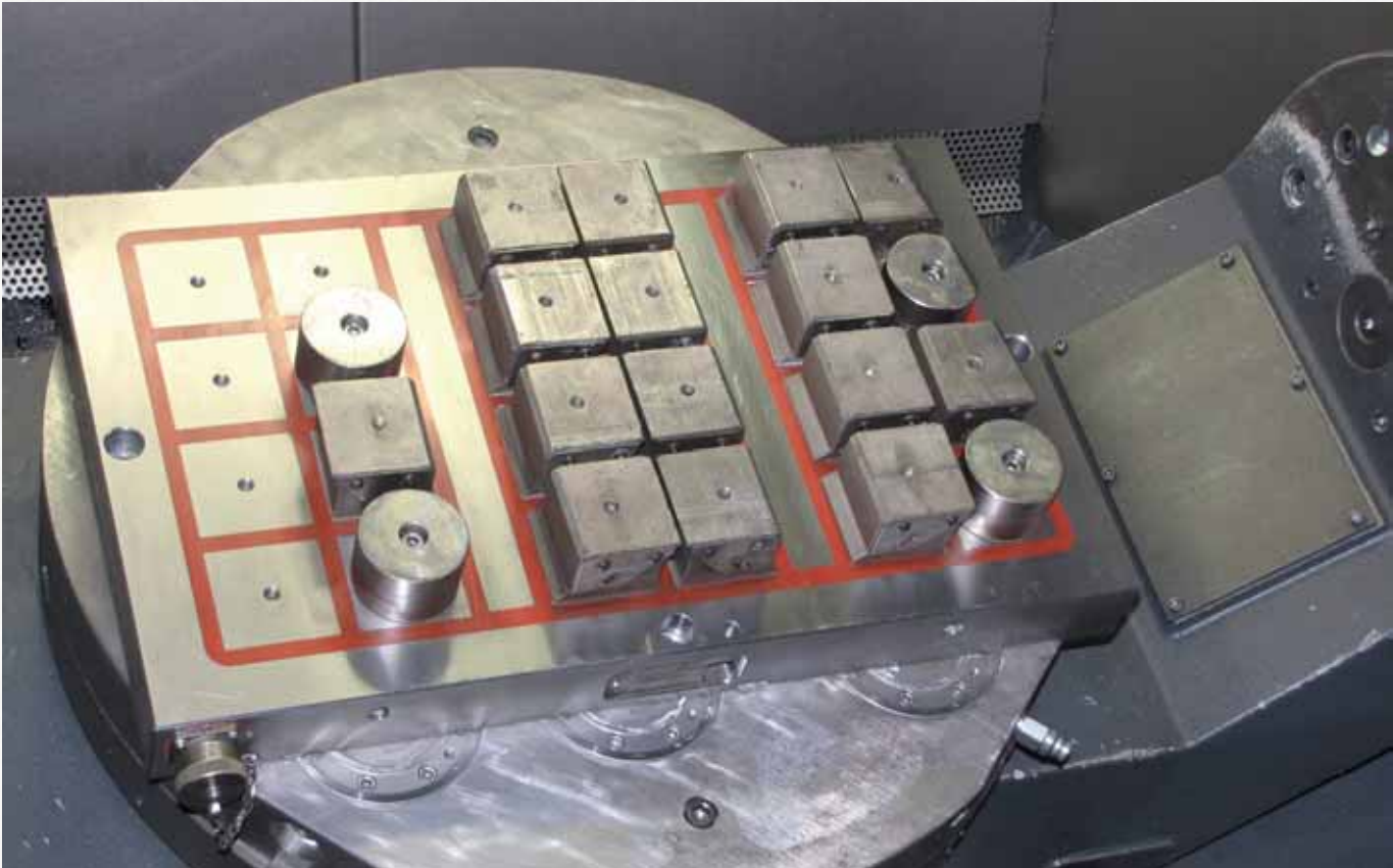
The Zero-Point System used together with the AMF magnetic clamping technology With friendly recommendation of Bäuml CNC-Fertigungs-GmbH & Co. KG, Weiden
