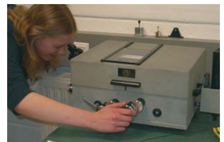
Verification by means of the interference comparator at the KOBA laboratory.
